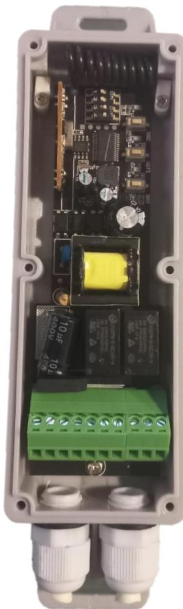
Central for tubular motor with power supply 110 - 240 V. With function OPEN/STOP/CLOSE available for AC switch and control remotes (frequency 433.92 - 868 MHz).
